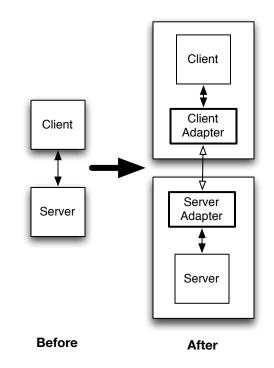
Figure 5.7: Architecture of the Connection Adapters
