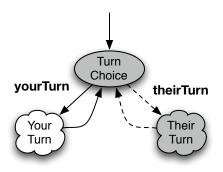
Figure 5.6: The protocol diagram for the role choice pattern.
