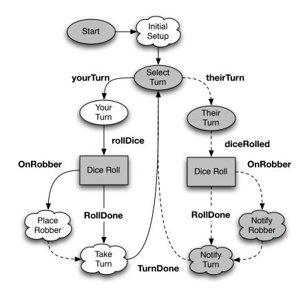
Figure 5.8: An Overview of the Server/Client Protocol for JSettlers.
