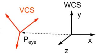
$$M_{cam} = \begin{bmatrix} 1 & 0 & 0 & P_{eye,x} \\ 0 & 1 & 0 & P_{eye,y} \\ 0 & 0 & 1 & P_{eye,z} \\ 0 & 0 & 0 & 1 \end{bmatrix} \begin{bmatrix} i_x & j_x & k_x & 0 \\ i_y & j_y & k_y & 0 \\ i_z & j_z & k_z & 0 \\ 0 & 0 & 0 & 1 \end{bmatrix}$$
