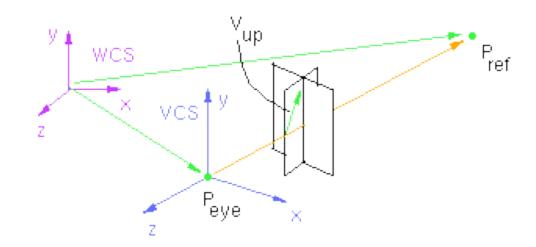
To build Mcam we need to define a camera coordinate system (origin, i, j, k)
