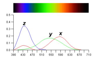
If we are given a spectrum and wish to find the corresponding X, Y, and Z quantities, we can do so by integrating the product of the spectral power and each of the three matching curves over all wavelengths. The weights X,Y,Z form the three-dimensional CIE XYZ space, as shown below.
