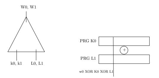
Suppose we have the circuit as above. We take PRG K0 and PRG L1 and now we bitwise XOR the first portion of both PRGs. We write W0 XOR K0 XOR L1. We can use different sections of the PRG to encrypt other combinations.
