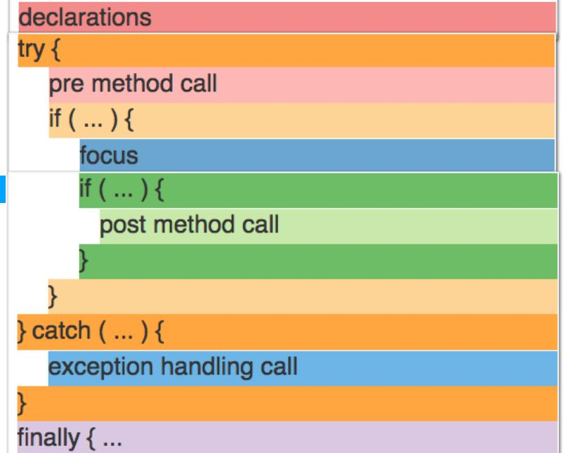
The diagram illustrates the structure of an API skeleton using colored horizontal bars. The bars are grouped into sections: declarations (red), try (orange), if (light orange), focus (blue), if (green), post method call (light green), } (green), catch (orange), exception handling call (light blue), } (orange), and finally (purple). The text within each bar corresponds to the code blocks shown in the code snippet above.
