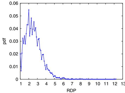
Fig. 8. Distribution of RDP in a HMTP tree of 100 members.
