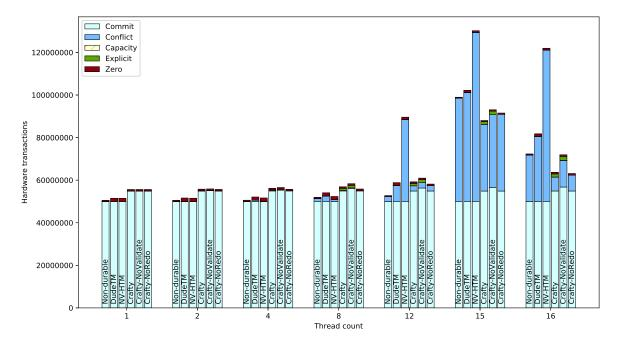
Figure 13. Persistent and hardware transaction breakdowns for the B+ tree microbenchmark with mixed operations.
