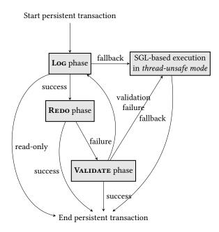
**Figure 3.** Crafty's phases in *thread-safe* mode.
