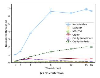
**Figure 6.** Throughput of Crafty and competing approaches, using the bank microbenchmark at three contention levels. Crafty generally outperforms NV-HTM and DudeTM, especially under low contention and at low thread counts.
