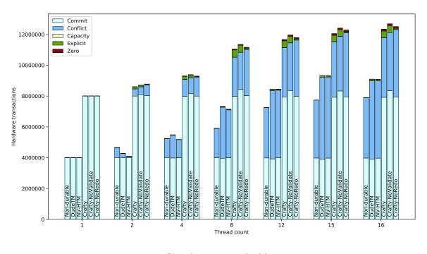
Figure 9. Persistent and hardware transaction breakdowns for the bank microbenchmark (high contention).
