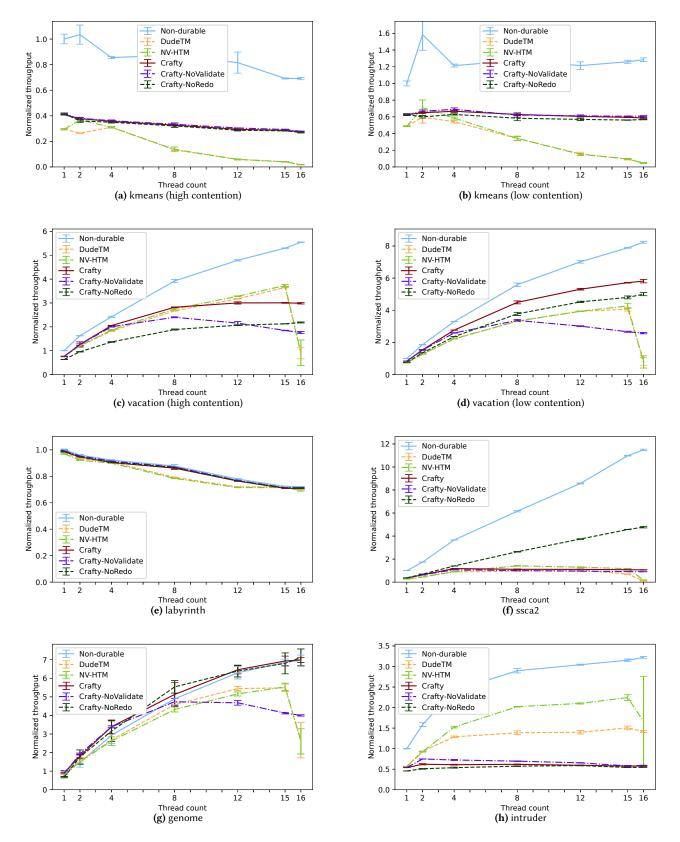
**Figure 8.** Throughput of Crafty and competing approaches, on the STAMP benchmarks. Crafty has low overhead and scales well at high thread counts.
