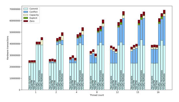
Figure 21. Persistent and hardware transaction breakdowns for intruder.
