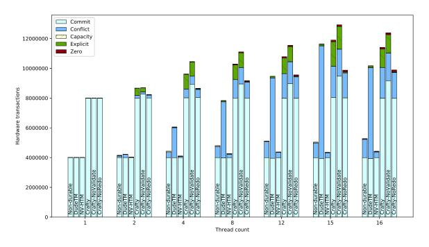
Figure 10. Persistent and hardware transaction breakdowns for the bank microbenchmark (medium contention).
