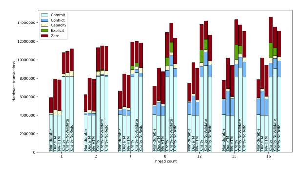
Figure 17. Persistent and hardware transaction breakdowns for vacation (low contention).
