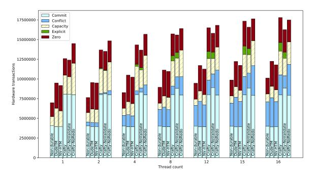
Figure 16. Persistent and hardware transaction breakdowns for vacation (high contention).
