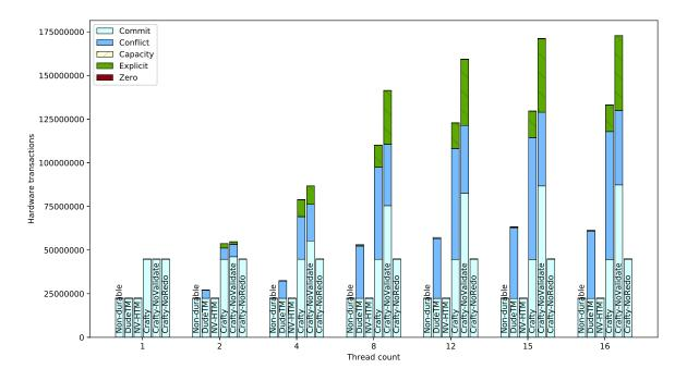
Figure 19. Persistent and hardware transaction breakdowns for ssca2.
