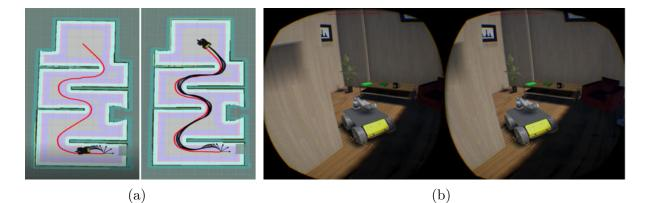
Figure 5.6: VRGym-ROS bridge. (a) The robot navigation in the scene imported into the Gazebo, exported from the VRGym. The red curve indicates the path planned by the robot's global planner. The black curve is the actual trajectory executed by the robot. (b) A Husky-UR5 robot is imported into VRGym from ROS to guide the way and open the door for a human agent.
