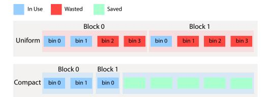
Figure 3.8: **Compact storage.** Particles are often unequally distributed in space. Hence, uniformly allocating fixed memory space for each particle block would result in a significant amount of unused memory. Instead, a more efficient strategy is to allocate just enough particle bins for each block according to the current distribution of particles.
