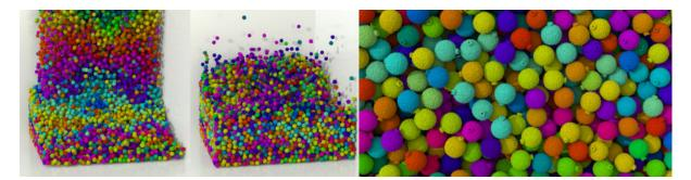
Figure 3.2: **Bomb falling.** We run the *bomb falling* test on 8 GPUs with 134M particles (6,688 bombs with nonlinear finite-strain hyperelastic constitutive models) and grid resolution  $512 \times 2048 \times 512$ . On average, each frame is finished within 1 minute, indicating the scalability of our proposed multi-GPU MPM pipeline.
