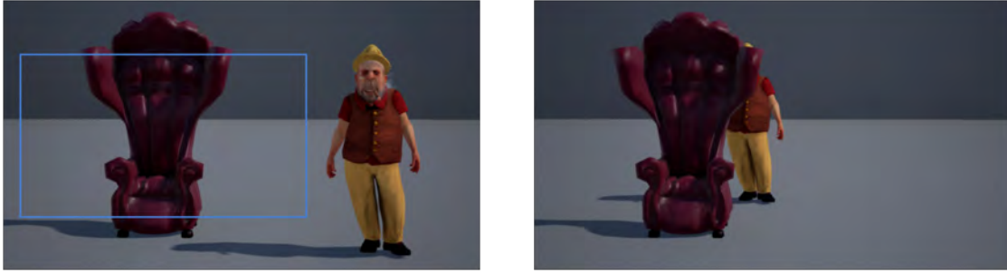
Figure 7.4: Illustration of the two types of visibility consideration. In the left image, if the frame is cropped to be within the bounds of the blue rectangle, the character will be beyond the frame bounds and therefore not visible. In the right image, the camera's view of the character is mostly occluded by the chair and the character is therefore not visible. The character is only visible if they are within the bounds of the frame and not occluded.
