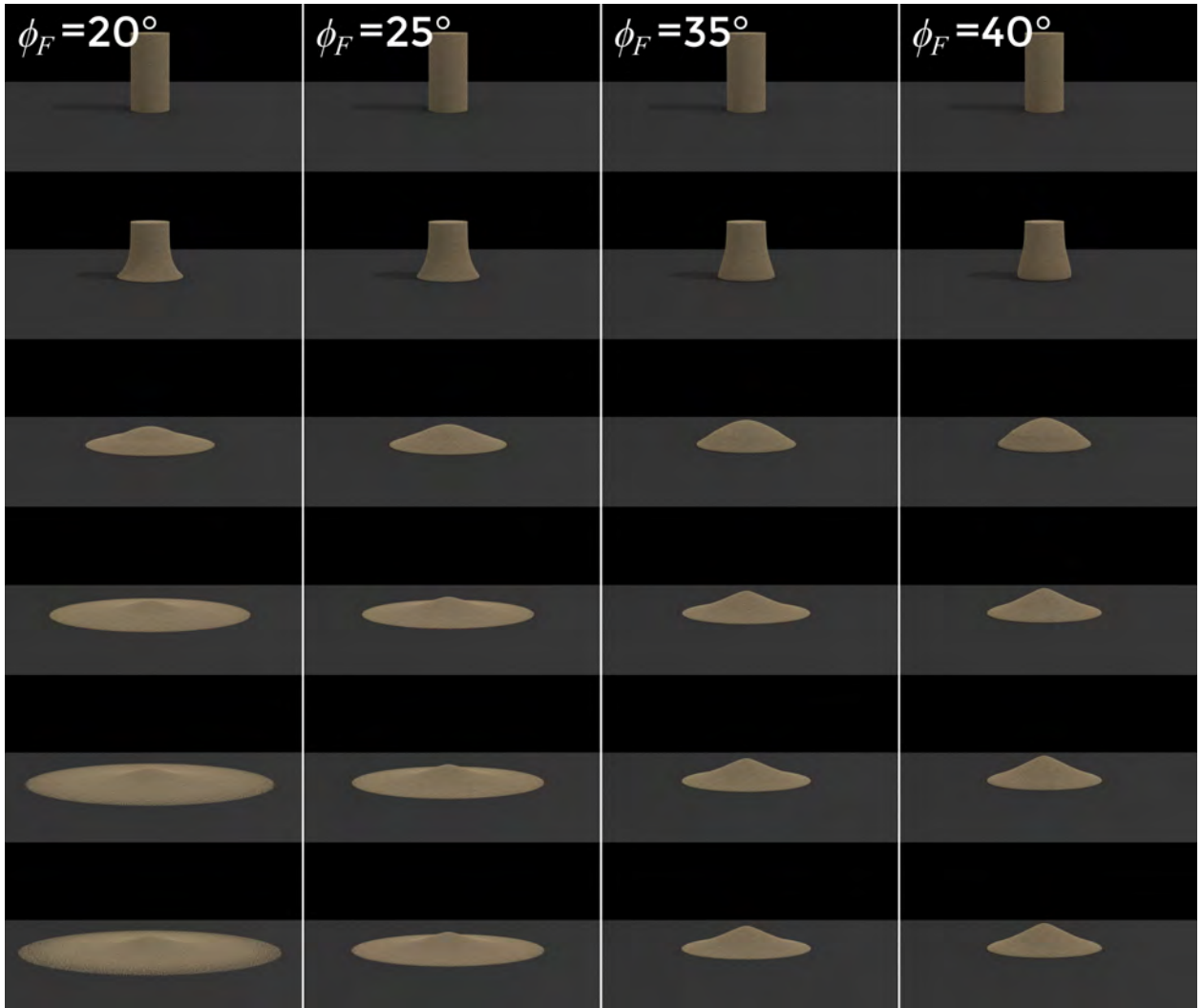
Figure 4.1: Effect of friction angle on piling.
