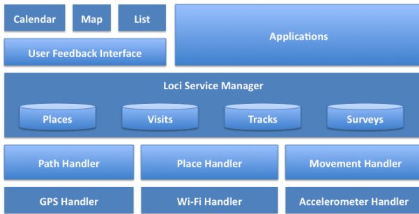
Figure 1. Loci semantic location service architecture
