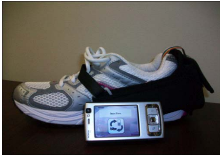
Figure 5. The complete wearable SmartShoe system. The Nokia n95 is pictures here running a mobile SmartShoe application built upon HIP's framework. Gait parameters are calculated in real time using a custom HIP module. HIP facilitates communication between embedded processors within the shoe as well as health care professionals via WiFi, GSM, and text messaging services.
