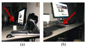
Figure 11. Experimental setup for monitoring browsing activity using ambient light sensors; with (a) the tablet placed on a 10cm platform centered in front of the screen; and (b) the tablet placed on the table to the left of the screen.
