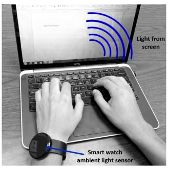
Figure 1. LuxLeak attack model overview, where smart device ambient light sensors are used for capturing screen emanations for monitoring computing activity.
