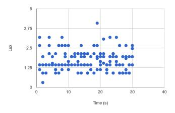
Figure 6. Scatter plot of the lux reading values for the letter 'D'. The 1<sup>st</sup> 10 seconds and 3rd 10 seconds show the readings as the number is being typed. The  $2^{nd}$  10 seconds show the readings as the hand returns to the home keys.
