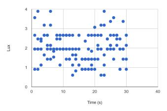
Figure 5. Scatter plot of the lux readings for the number '9'. The  $1^{st}$  10 seconds and 3rd 10 seconds show the readings as the number is being typed. The  $2^{nd}$  10 seconds show the readings as the hand returns to the home keys.
