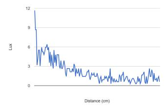
Figure 4. Lux values as distance from screen is increased 1 cm per second for 30 seconds, averaged over 3 runs. The Moto360 smart watch was positioned with its face perpendicular to the screen.
