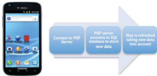
Figure 7 | Interfacing between the android device and PHP script that allows for all users' information to be displayed on a collective map.
