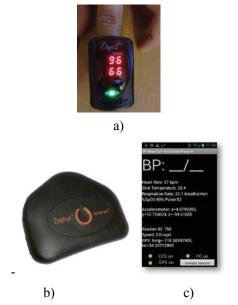
Figure 3. Virtual Cuff Sensor and Interface. a) Nonin Onyx II 9560 Fingertip Pulse Oximeter used on the finger to derive PPG signals. b) Zephyr Bioharness strapped to the users chest collects ECG data. c) Screen Shot of Android App
