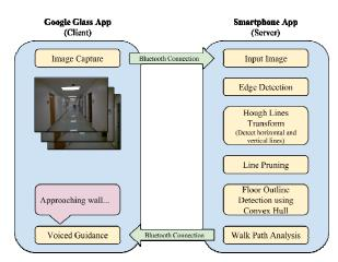
Figure 3. The Google Glass app provides the input and output information from and to the user. The Smartphone app performs Floor Extraction and Analysis by performing a series of image processing algorithms.
