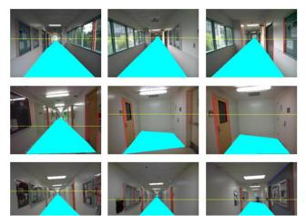
Figure 8. The floor detection algorithm is able to estimate the floor region from captured images of corridors with different color, texture, and lighting. The images above shows the results of the floor detection phase from different datasets.
