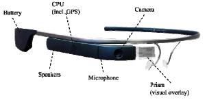
Figure 1. Google Glass is a rechargeable batteryoperated wearable device with built-in features such as camera, speakers, Bluetooth, Wi-Fi, etc. accessible for most people. The higher processing power and better battery life in these smartphones as compared to Google Glass allows for an ideal mobile and lightweight device for performing powerful operations that might prove difficult to run on the Glass.
