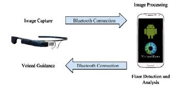
Figure 2. Images captured by the Google Glass are sent over to the Android smartphone via Bluetooth for Image Processing and Floor Detection and Analysis. The results of the analysis are sent back to the Google Glass for voiced guidance.
