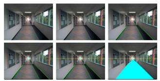
Figure 4. Results of each image processing step. From topbottom, left-right: (a) input image, (b) vertical lines in red, (c) horizontal lines in green, (d) cyan dots as the intersections of every pair of horizontal lines (vanishing point), (e) yellow line as the average y-axis value of all vanishing points, (f) convex hull of detected horizontal lines.
