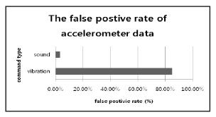
Fig 4.3 The false positive rate of accelerometer data with and without vibration command
