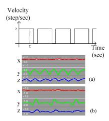
Fig 3.7. Scheduled interval training and the accelerometer data for the accurate exercise (a) and the inaccurate exercise (b) at time t
