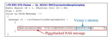
Fig. 6. The RRC layer helps to deliver NAS message when RRC protocol interacts with NAS protocol
