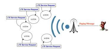
Fig. 13. The paging broadcast message can be used to drain batteries of multiple devices
