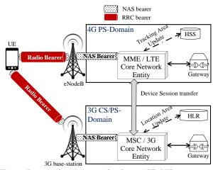
Fig. 2. Inter-radio access technologies (IRAT) interaction
