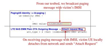
Fig. 10. The network and UE logs show that the paging message with victim's IMSI can detach the victim device from the network
