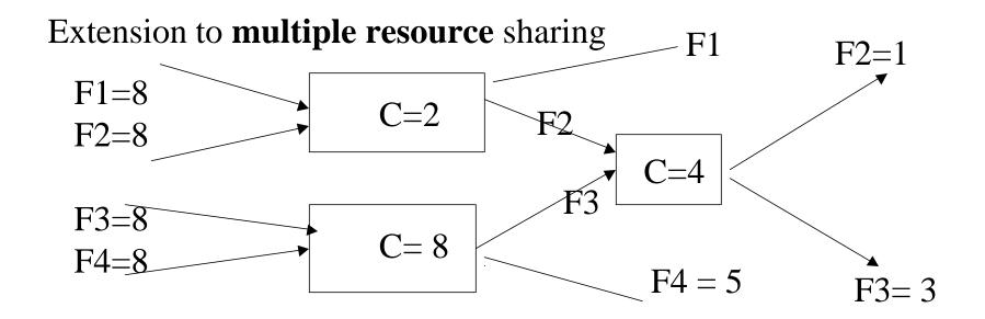
Iterative construction approach (given the routing):
