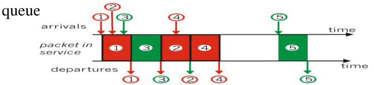
• Weighted Round Robin: is a generalized Round Robin in which an attempt is made to provide a class with a differentiated (ie **different weight** eg based on pkt size) amount of service over a given period of time
