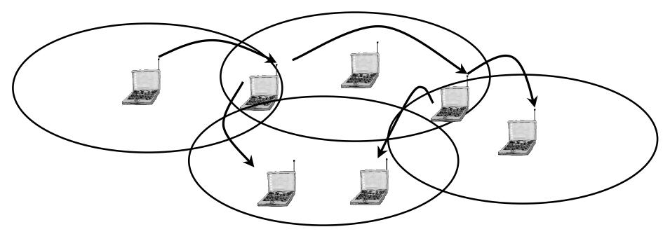
Tree-based protocols not applicable due to dynamic topology Flooding highly inefficient with high degree of connectivity (n transmissions instead of 1)
