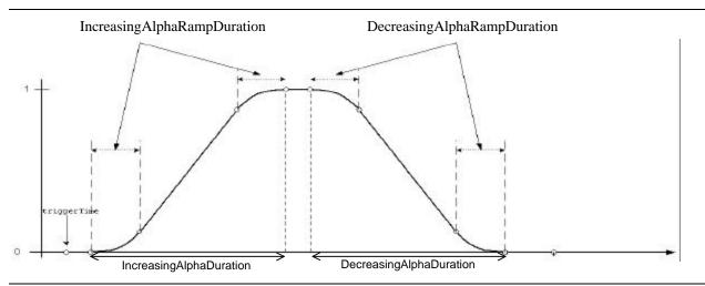
Figure 5-6 Smoothing of the Waveform Produced by Alpha<sup>9</sup>
