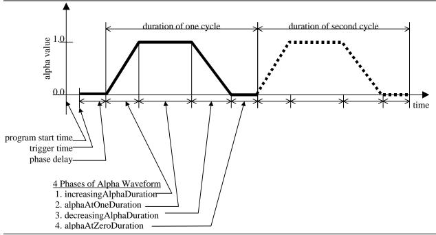
Figure 5-2 Phases of the Alpha Waveform.
