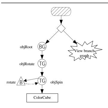
Figure 1-20 Scene Graph for HelloJava3Dd Example
