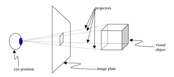
Figure 1-9 Conceptual Drawing of Image Plate and Eye Position in a Virtual Universe.
