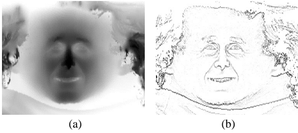
Figure 3: (a) Original range map. (b) Modified Laplacian field function of (a).
