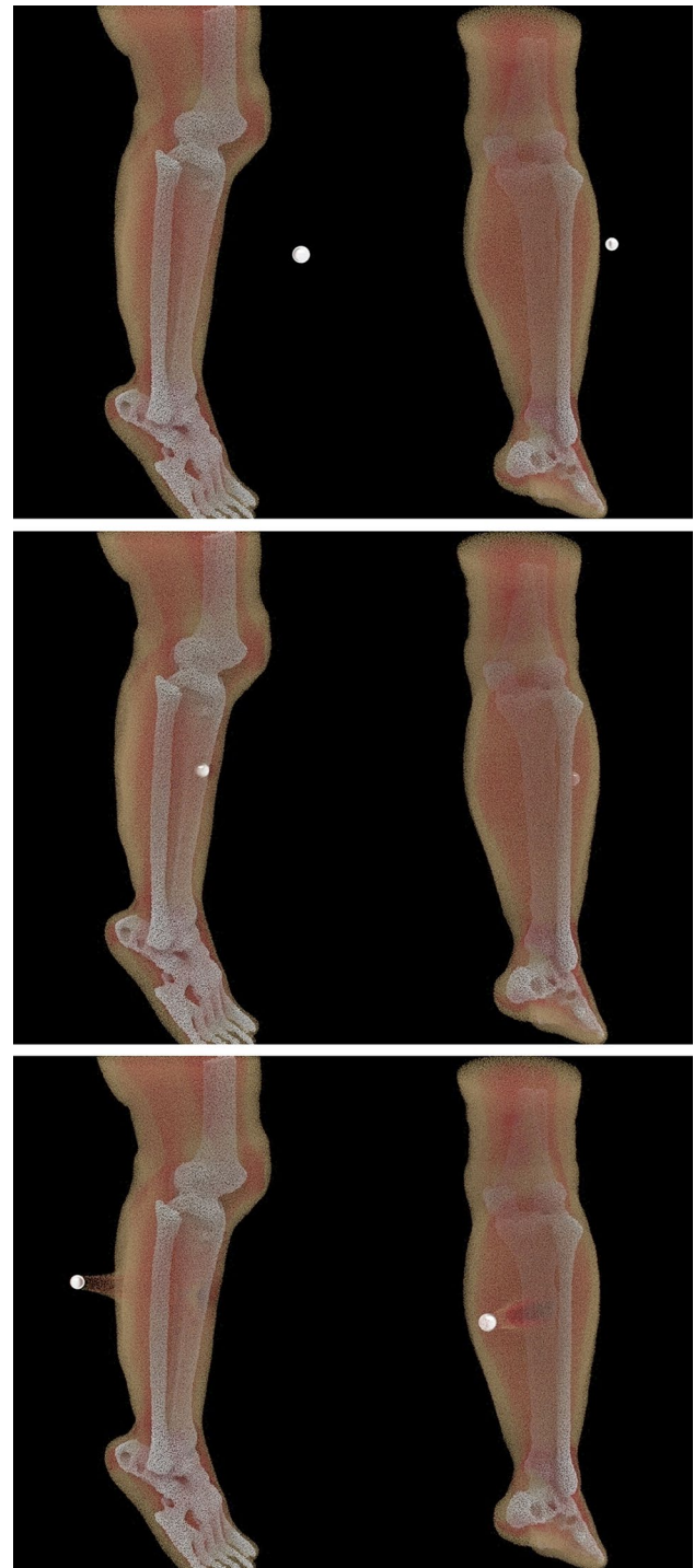
Fig. 2 Material point method (MPM) simulation of projectile impact. Yellow, red and white particles represent skin, tissue and bone, respectively. The first column shows the side view and the second column shows the back view (color figure online)
