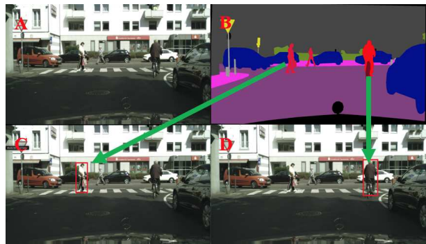
Figure 1. An example of ground truth bounding box generation. A) An original image provided by the CITYSCAPES dataset; B) A corresponding image with segmentation masks provided by the CITYSCAPES dataset; C) a 'Person' with bounding box generated from the segmentation mask; D) a 'Rider' with bounding box generated from the segmentation mask.
