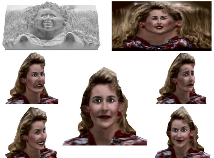
Plate 1: Objective. Input : Range map in 3D and texture map (top). Output : Functional face model for animation.
